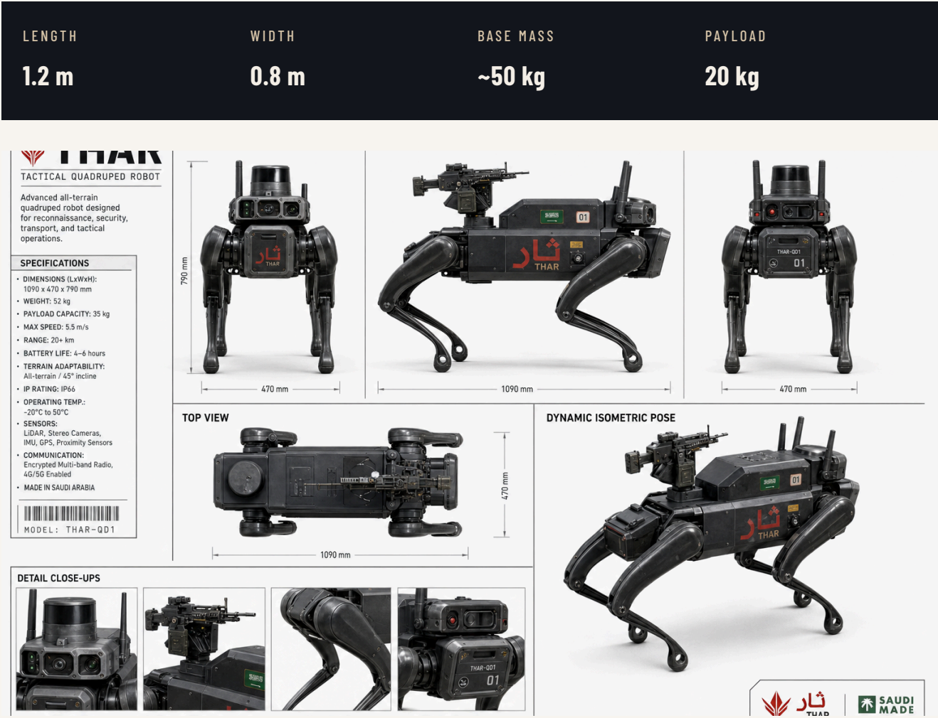
FIG 1.1 DYNAMIC POSE SHEET — STANCE ADAPTATION AND PAYLOAD BALANCE ACROSS MISSION PROFILES
